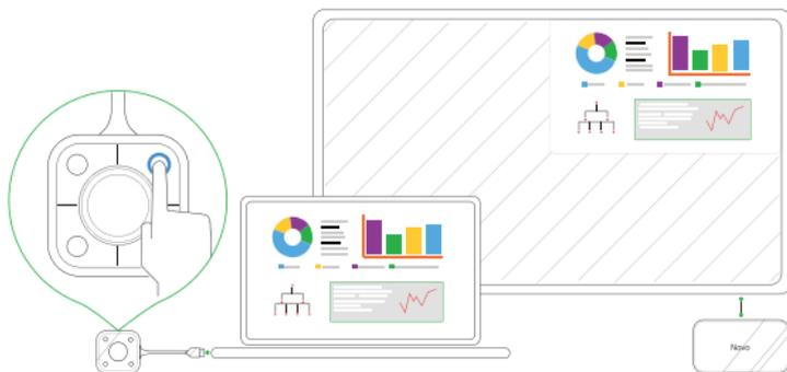
⑧ Press any corner button on the LauncherPlus to project your computer's screen onto the corresponding quadrant of the display, the button's blue LED will light when it is in use.
