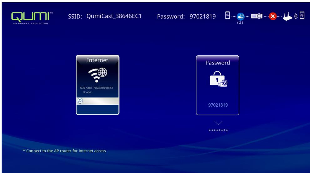
12. Press the ▲ or ▼ on the remote or smart device to select a listed SSID and press ←.
